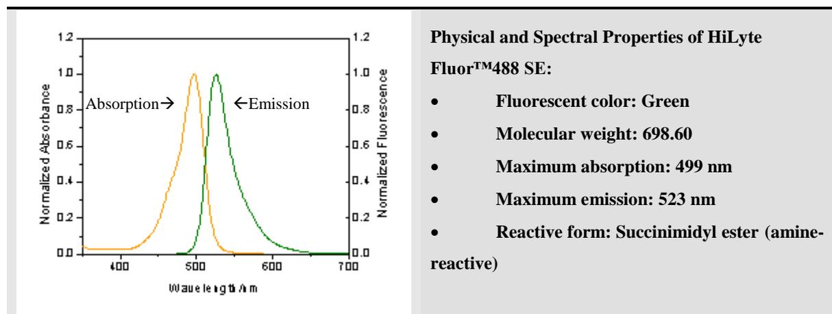
HiLyte Fluor™ 488 SE is an excellent amine-reactive fluorescent labeling dye for generating protein conjugates. The spectrum of HiLyte Fluor™ 488 is similar to fluorescein (FITC), resulting in an optimal match to filters designed for fluorescein. More photostable than FITC, HiLyte Fluor™ 488-labeled proteins allow additional time for capturing image.
