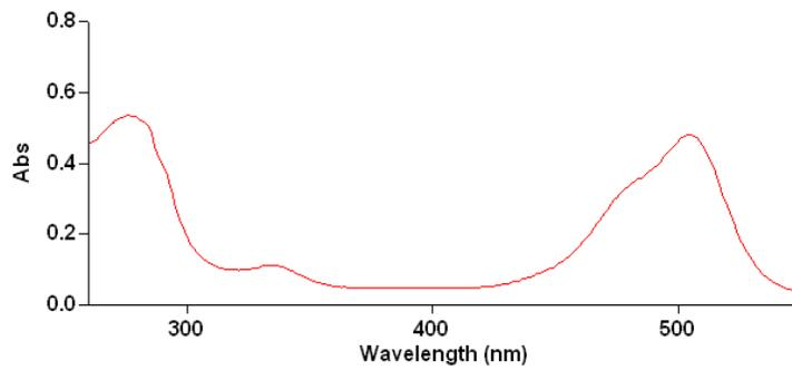
Figure 2. The absorbance spectrum of HiLyte Fluor™488-Ig G conjugate.
